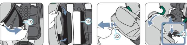
5. Open the two shoulder cushions (19) by the Velcro fasteners on the side.
