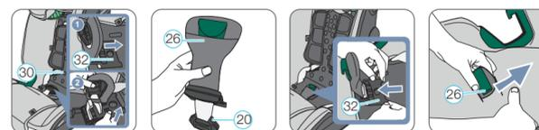
9. Raise the grey release plate (32) and push it along with the harness buckle (20) towards the backrest (30).
