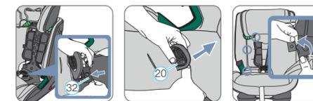
12. Store the SecureGuard (26) in the recess provided and push the grey release plate (32) back into its holder until it engages with an audible click.
